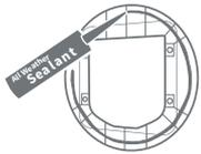
4 We recommend running a bead of 'All Weather Sealant' around the edge of the mounting adaptor for both sides of the glass. The sealant will help secure the pet door in place after installation, particularly with larger hole sizes, and also help prevent moisture getting in from outside. This type of sealant can be purchased from a glazing company and most DIY stores.
