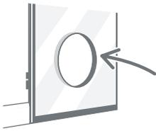
3 If installing the SureFlap Microchip Pet Door in a double glazed panel your glazier should seal between the panels around the circular hole to avoid moisture collecting inside. Do not use metal in any such seal.
