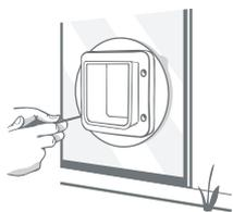
8 Screw the two halves together. If mounting in a single pane use the shortest of the three pairs of screws. A double glazed panel may require the mid-sized screw, depending on its thickness. Check the assembly is centred with the circular hole before fully tightening the screws.
