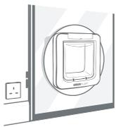
6 From inside of the house, slide the tunnel of the main assembly through the hole in the glass.
