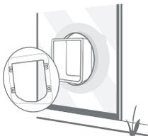
7 From outside of the house, mount the second part of the mounting adaptor and then the external frame.
