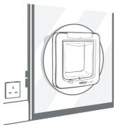
6 From the inside of the house, slide the tunnel of the main assembly through the hole in the glass.
